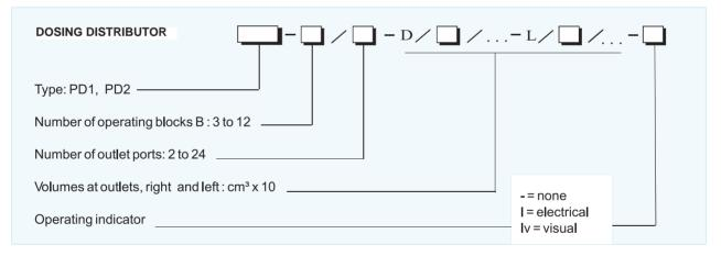
**NOTE:** Installing interconnection results in the volume which is the total of individual volumes. The flow rate is equal to zero if the screw "X" is removed and an outlet port is pluged. Complete volume is directed through the port on the opposite side.
