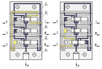
the lubricant is supplied to distributor. There are various possibilities of combining outlet volumes. Removing the screw "X" and pluging an outlet port results in duplicating the lubricant quantity on the opposite outlet port. Interconnecting the neighboring blocks results in summation of their outlet volumes.
